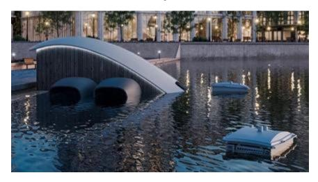
A swarm of RanMarine ASVs operating out of a shared SharkPod docking station enables fully-automated waste removal coverage of a water area, on a 24x7 basis. This results in significant operational cost savings through reduced labor cost, while delivering simultaneous increases in both productivity and data quality.
